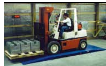
20,000 LB. CAPACITY SCALE SHOWN WITH OPTIONAL APPROACH RAMPS. CONTACT FACTORY FOR RAMP INFORMATION.
