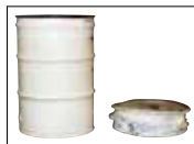
Crushes 55 gallon steel drums to only 6" high.
