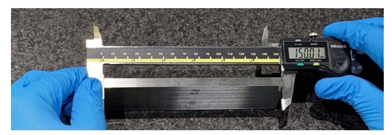
Caliper calibration using gage blocks
