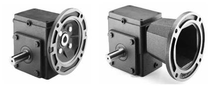
At left, a quill-style input worm gear reducer uses a hollow input shaft and a shallow mounting flange. At right, extended mounting flange accommodates a solid-shaft to solid-shaft input with a flexible coupling joining the two shafts.
