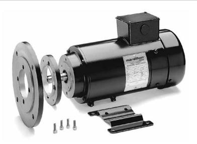
Three common IEC mounting options are shown in this photo. From left, a B5 flange, B14 face and rigid B3 base. In this case, any of the options can be bolted to a modularly designed round-body IEC 71 frame motor.
