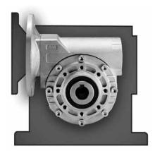
Graphic shows compact size of an aluminum-housed worm gear reducer compared with a cast iron housed reducer of the same center distance. Smaller size and lighter weight can be an application advantage in many cases, but reduced mass means that the reducer's thermal rating must be carefully considered.
