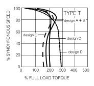
**Polyphase** induction motors have a high starting torque, power factor, high efficiency, and low current. They do not use a switch, capacitor, relays, etc., and are suitable for larger commercial and industrial applications.
