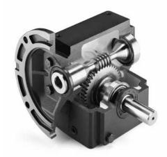
Cutaway view shows key components of an industrial-duty worm gear reducer. Note steel worm and bronze worm gear. Seals on both input and output shafts prevent lubricant leakage.
