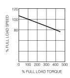
Both designs have linear speedtorque characteristics over the entire speed range. SCR rated motors – those designed for use with common solid-state speed controls – feature high starting torque for heavy load applications and reversing capabilities, and complementary active material to compensate for the additional heating caused by the rectified AC input. Designs are also available for use on generated low-voltage DC power or remote applications requiring battery power.
