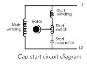
Moderate-torque motors are used on applications in which starting requires torques of 175% or less or on light loads such as fans, blowers, and light-start pumps. High-torque motors have starting torques in excess of 300% of full load and are used on compressors, industrial, commercial and farm equipment. Capacitor start motors use a start capacitor and a start switch, which takes the capacitor and start winding out of the circuit when motor reaches approximately 75% of its operating speed.
