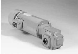
Three-phase NEMA C face AC motor combined with flanged worm gear reducer results in a "workhorse" industrial gearmotor. This straightforward mounting approach is common with motors ranging in sizes from fractional through 20 HP and larger.
