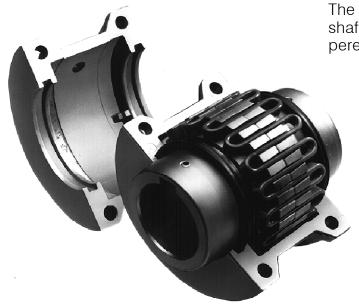
The basic GRID-LIGN coupling consists of two steel shaft hubs, a high strength spring steel tapered grid element, two seals and a cover as-
