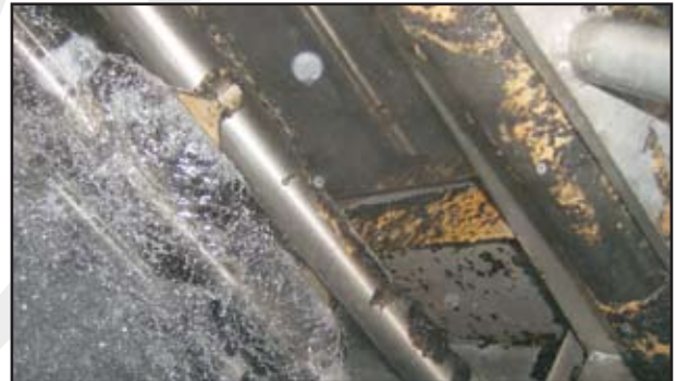
Typical Dead Zone above Nozzle Bed
