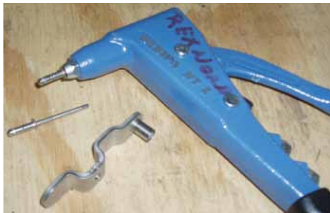
9200 Chain Rivet Tool, Clip and Stainless Steel Rivet
