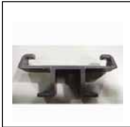
Evidence of uneven wear on top plate
