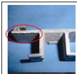
Evidence of obstruction – bent TABs
