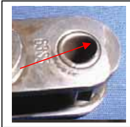
Evidence of overload – deformed bushing
