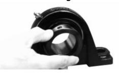
The inner ring of the bearing is locked to the shaft by a quarter-turn of the eccentric collar in the direction of shaft rotation. The collar is secured in place with a single setscrew.
