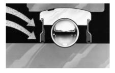
PROGUARD positive contact low drag seal DODGE SXR/SXV/SLX mounted ball bearings use the PROGUARD land-riding contact seal with steel shield protection. This highly effective, positive seal design assures uniform lip contact with the inner ring to seal out contaminants and seal in lubricants.
