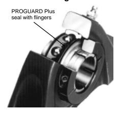
On SXR bearings, optional flingers can be added to form a tight labyrinth with the PROGUARD Seal and provide additional seal protection against contaminants and debris.
