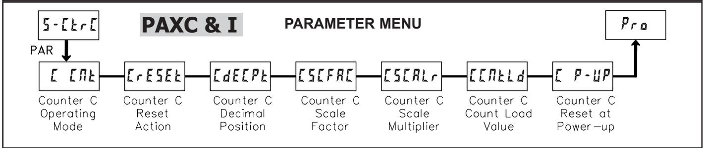
Module 5 is the programming for Counter C. For maximum input frequency, the counter operating mode should be set to *none* when not in use. When set to *none* the remaining related parameters are not accessible. The C annunciator indicates that Counter C is being shown in the Display Mode. An Exchange Parameter List feature for scale factor and count load values is explained in Module 2.
