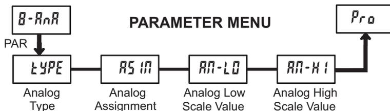
Module 8 is the programming for the analog output parameters. To have an analog output signal, an analog output option card needs to be installed (See Ordering Information). For analog output hardware and wiring details, refer to the bulletin shipped with the option card.
