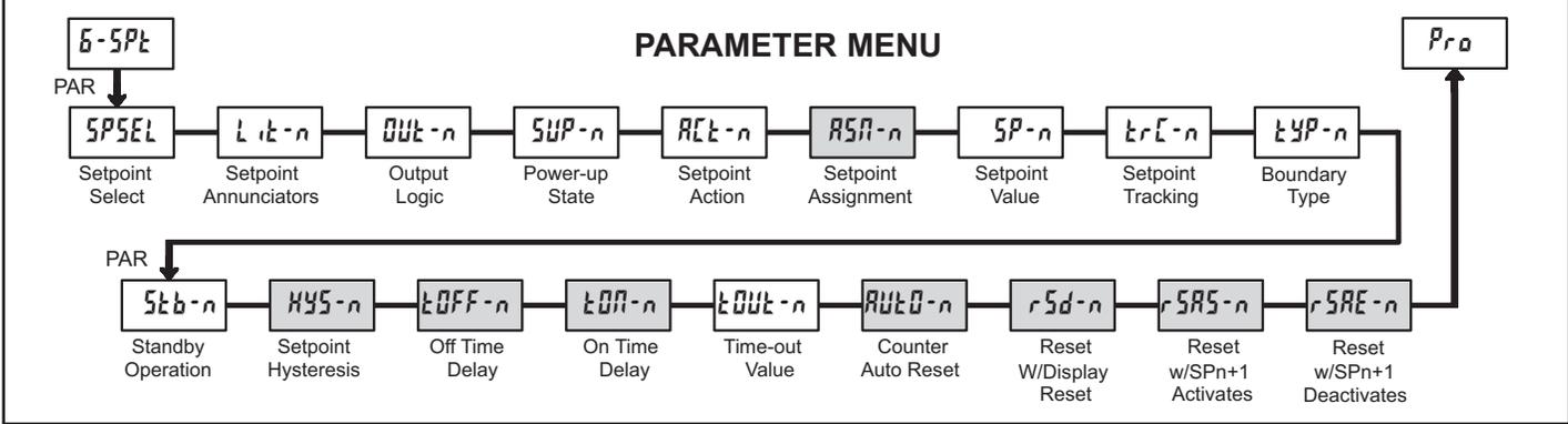
Module 6 is the programming for the setpoint (alarms) output parameters. To have setpoint outputs, a setpoint option card needs to be installed into the PAX (see Ordering Information). Depending on the card installed, there will be two or four setpoint outputs available. For setpoint hardware and wiring details, refer to the bulletin shipped with the option card. For maximum input frequency, unused Setpoints should be configured for **OFF** action.
