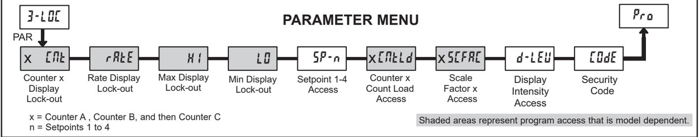
Module 3 is the programming for Display lock-out and “Full” and “Quick” Program lock-out.
