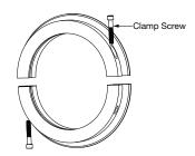
Figure 22 - Oil Seal Assembly (O-ring not shown)
