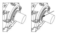
Figure 38 - Auxiliary Seal and Retainer
