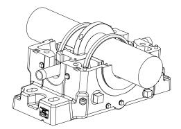
Figure 13 - Oil Rings Installed
