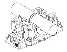
Figure 8 - Liner Base Installed
