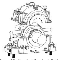
Figure 27 - Housing Cap Installation
