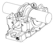
Figure 14 - Retainer Washer Installation
