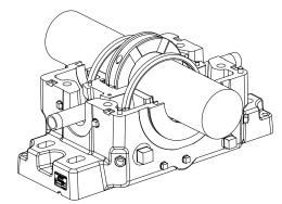
Figure 17 - Thrust Plates Installed
