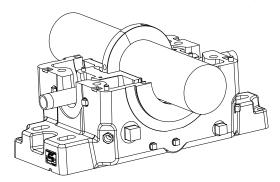
Figure 10 - Thrust Collar Installed
