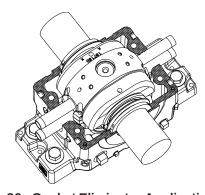
Figure 26 - Gasket Eliminator Application Area
