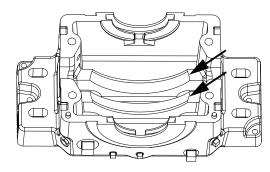
Figure 6 - Spherical Seats
