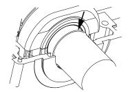
Figure 23 - O-ring Installation
