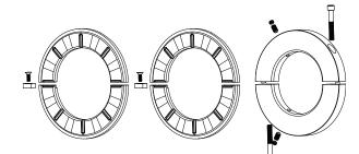
Figure 3 - Thrust Plates and Split Thrust Collar
