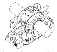
Figure 19 - Liner Cap Installation
