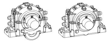
Figure 39 - Auxiliary Seal Housing
