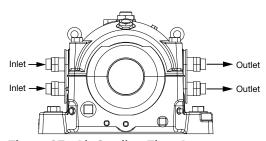
Figure 37 - Air Cooling Flow Arrangement
