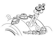
Figure 32 - Circulating Oil Inlet Kit Installation
