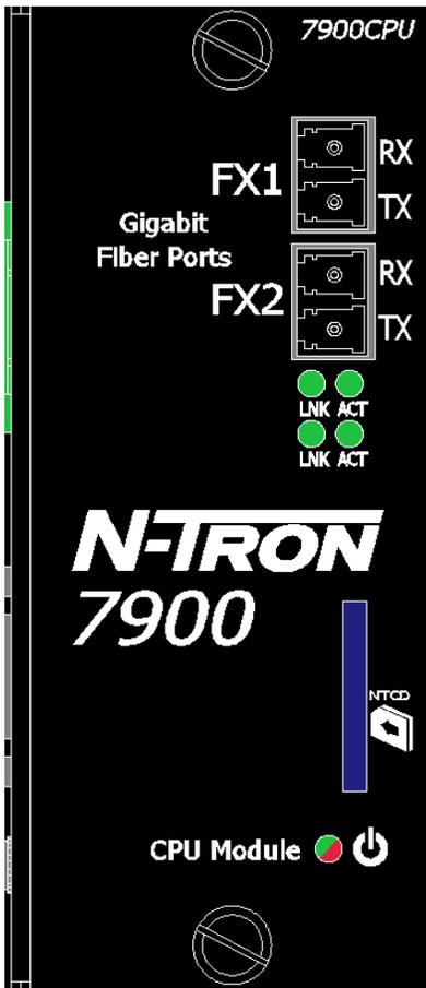
The configuration device is inserted into the front of the 7900 CPU Module.
