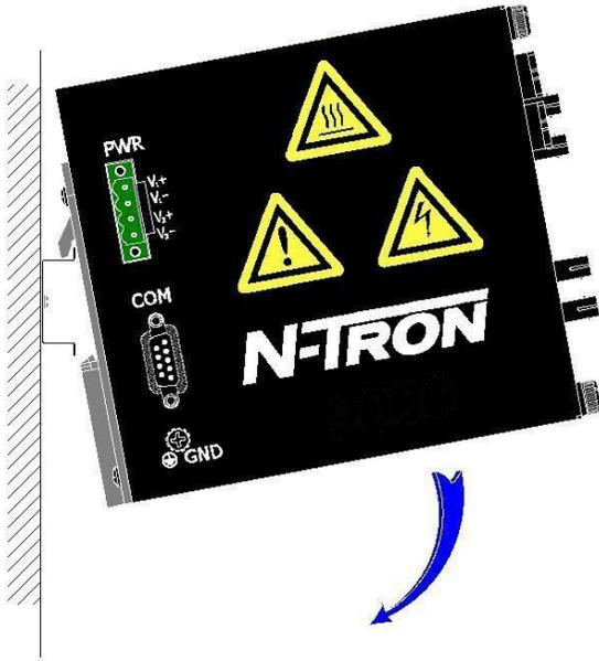
To mount the unit to the 35mm din-rail, place top edge of the bracket on the back of the unit against the din-rail at a 45° upward angle. Lower the bottom of the unit until it snaps into place.
