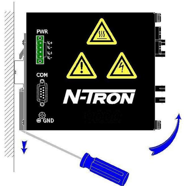
To remove the unit from the 35mm din-rail, place a flat head screwdriver into the release clip at the bottom of the unit, and push down on the clip until it disengages from the bottom of the unit from the din-rail. Lift the bottom of the unit up at an approximate 45° upward angle to completely remove the unit.
