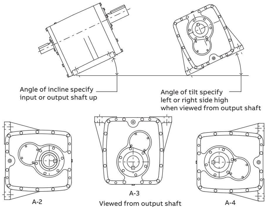
Dodge Maxum XTR concentric shaft reducers can be modified to permit mounting in positions other than the conventional (A-1) floor mounting. Some of these include ceiling (A-3) and wall (A-2 and A-4) and various inclined, vertical and tilted positions. Consult factory to determine what modifications are required for your specific application.
