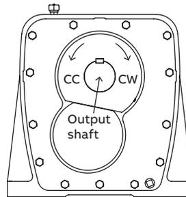
Backstop - specify direction of rotation of the output shaft (cw for clockwise, CC for counterclockwise) when looking toward the gearbox from the end of the output shaft
