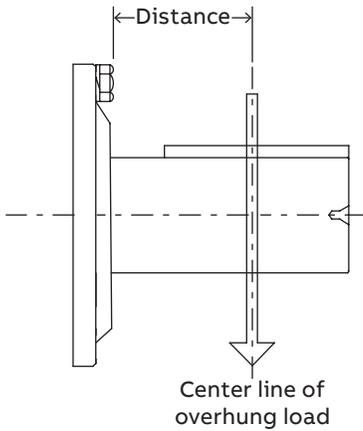
$$\text{OHL (lbs.)} = \frac{126,000 \times \text{Hp} \times \text{Fc} \times \text{Lf}}{\text{PD (inches)} \times \text{RPM}}$$
