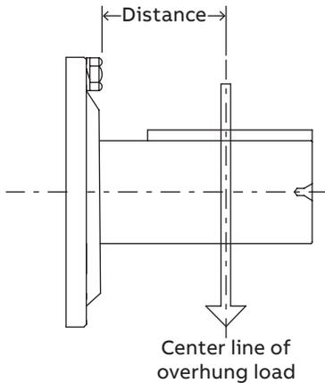
$$\text{OHL (lbs.)} = \frac{126,000 \times \text{Hp} \times \text{Fc}}{\text{PD (inches)} \times \text{RPM}}$$
