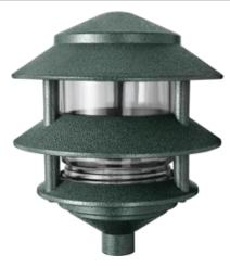
Rugged die cast aluminum 6" diameter housings. Threaded, gasketed clear glass globe for durable weatherproofing and easy relamping. 1" long, 1/2" threaded nipple included for easy mounting. 75 Watt max.
