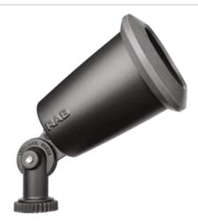
The economical R90 floodlight with a molded silicone external gasket to insure superior weatherproof seal. Polyester powder coating. PAR38 150 Watt max. Lamp not supplied.
