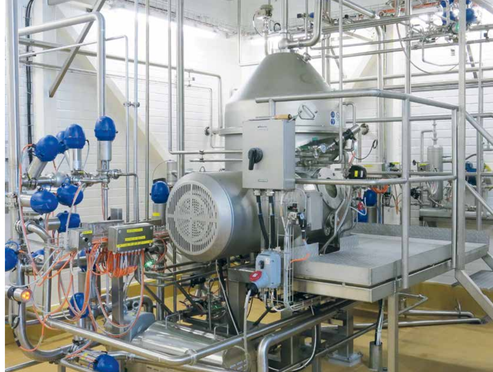
Valio's Seinäjoki plant produces all Valio quarks. A separator is used for producing quark. The pumps and mixers used by the separator are controlled by VACON® 100 AC drives. In recent years, quarks have been the quickest-growing product category in retail sales. Valio was able to quickly double its production at the Seinäjoki plant as butter production had recently moved to new premises.
