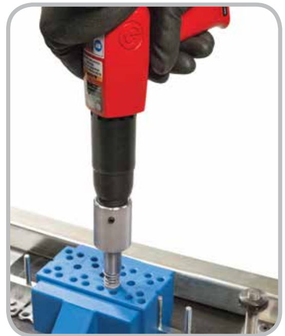
Air Powered Rivet Driver Installation
