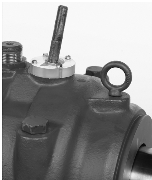
Figure 4 - PLXC Circulating Oil Inlet
