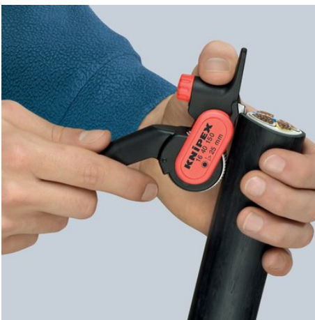
Setting the tool for longitudinal cut
