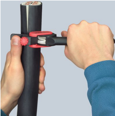
Turning the tool for circumferential cut
