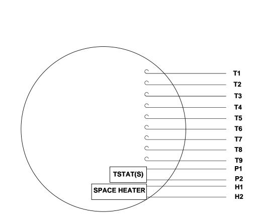
VIEW FROM OUTSIDE OF MOTOR AT SWITCH END. Uncontrolled Copy
