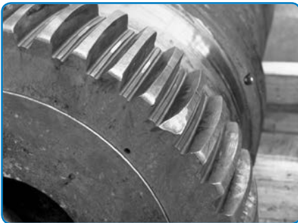
Tooth End Breakage due to over-misalignment
