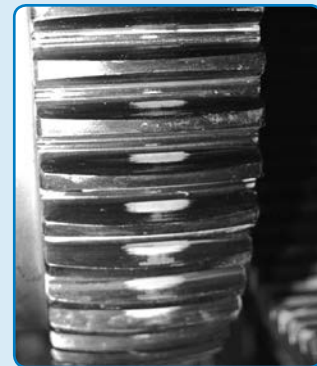
Carburized Gearing with blue contact check at 3° 20-40% gear teeth in contact
