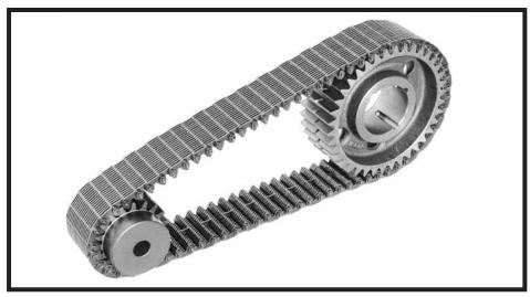
Morse® Silent Chain is an Inverted Tooth type drive offering particularly smooth, quiet power transmission at higher speeds up to 5000 FPM. The exclusive Morse Rocker Joint eliminates friction during chain articulation—permitting high rotative speed with less wear and heat.
