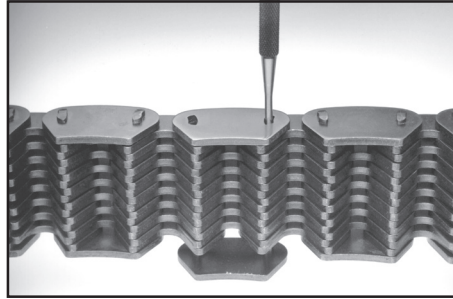
Fig. 2 Drive the two pins through the outside guide. Remove the outside guide and turn the chain over.
