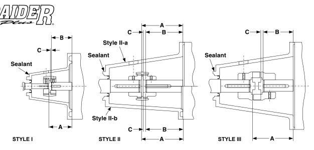
This kit is used to adapt a solid input shaft reducer to a C-flange motor. Place the reducer on a flat horizontal surface with the input up.
