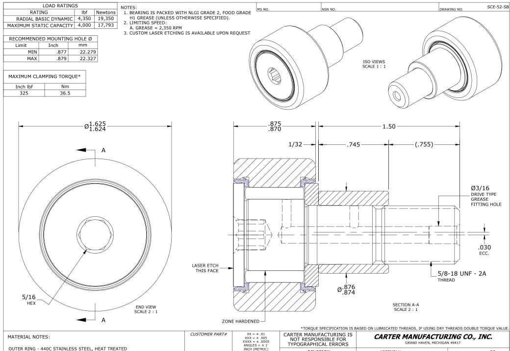
STUD - 440C STAINLESS STEEL, ZONE HARDENED WASHER - 440C STAINLESS STEEL, HEAT TREATED NEEDLE ROLLER(S) - 440C STAINLESS STEEL, HEAT TREATED SEAL(S) - SYNTHETIC
