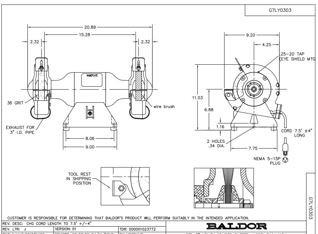
FILE: \AAA\00102\169 REVISED: 03:03:55 04/11/2017 BY: USGRHUR STD. 7" UTILITY GRINDER-BUFFER MODEL 34C 115V MTL: - $\bigcirc$ SH 1 of 1
