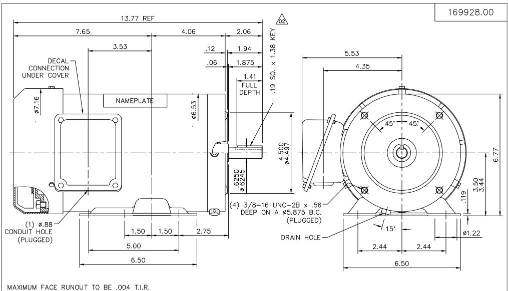
MAXIMUM FACE RUNOUT TO BE .004 T.I.R. MAXIMUM PILOT ECCENTRICITY .004 T.I.R. PERMISABLE SHAFT RUNOUT .002 T.I.R.
