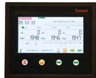
New Tsmart Touchscreen, showing new programming method/display.
