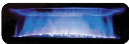
Axial Magnetic Field Interrupter - Arc Dispersion
