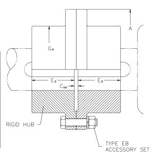
① LEF Discs are used only in close coupled applications. One disc is required per coupling. Note: For ratings and max. bores refer to page 134.
