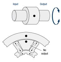
Any feedback torque from the output member is instantly stopped by the wedging of sprags between the fixed outer race and the output memberfeedback torque never reaches the control member.
