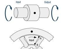
When input torque is reversed, the control member rotates a maximum of 6° to release the opposing set of sprags and then again drives the output member through point "B" on these sprags.
