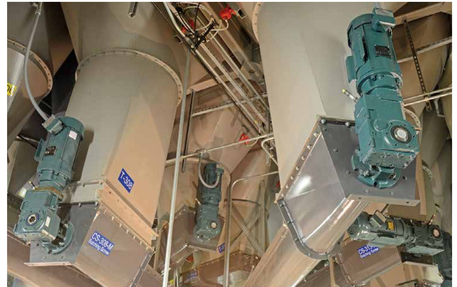
Screw Conveyor Corporation chose to use Baldor•Reliance explosion-proof motors and Baldor•Dodge Quantis Right-Angle Helical Bevel (RHB) reducers on the 15 batching screw conveyors. The motors are rated Division 1; Class I, Group D; and Class II, Group F & G, ensuring safety and reliability in a hazardous environment where combustible dust is present all or some of the time. RHB units were selected for their greater torque density in a compact housing.
