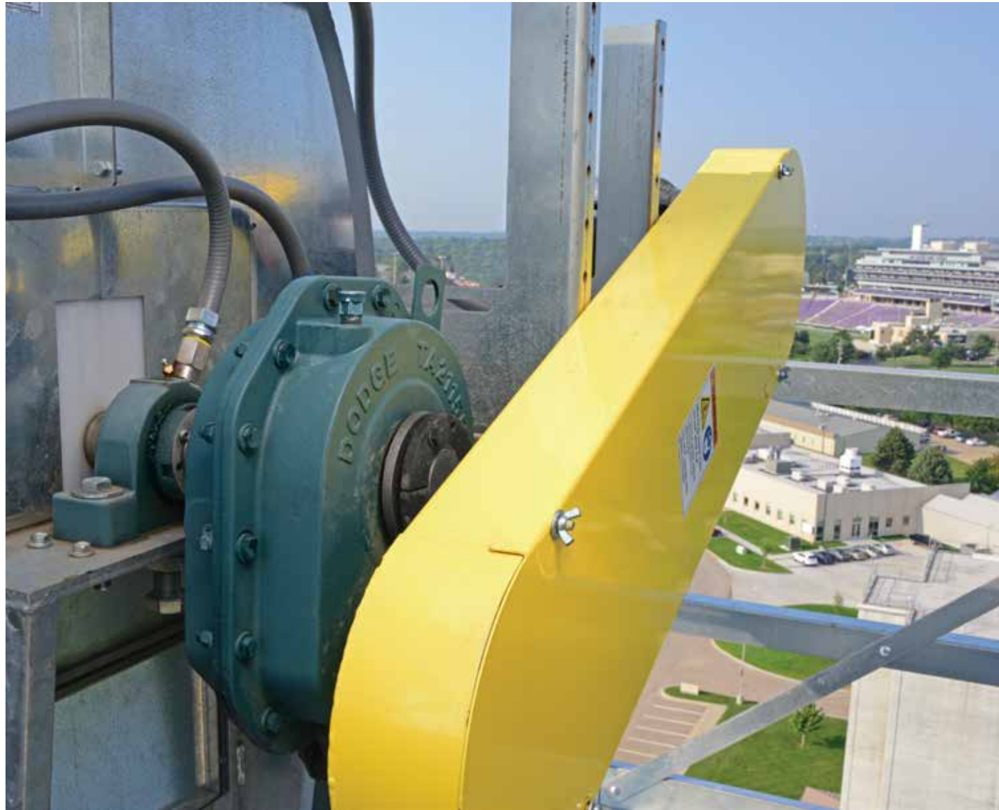
With more than 1.8 million units in service, Baldor's Dodge Torque-Arm II® gear reducers offer proven dependability and are the standard in the industry. This unit features the patented twin tapered bushing system that eliminates fretting corrosion and reducer wobble. Baldor's Dodge Imperial bearing, with its patented "push/pull" adapter system, was selected for its ease of installation. This bearing also features a patented sealing system, keeping lubrication in and contaminants out.
