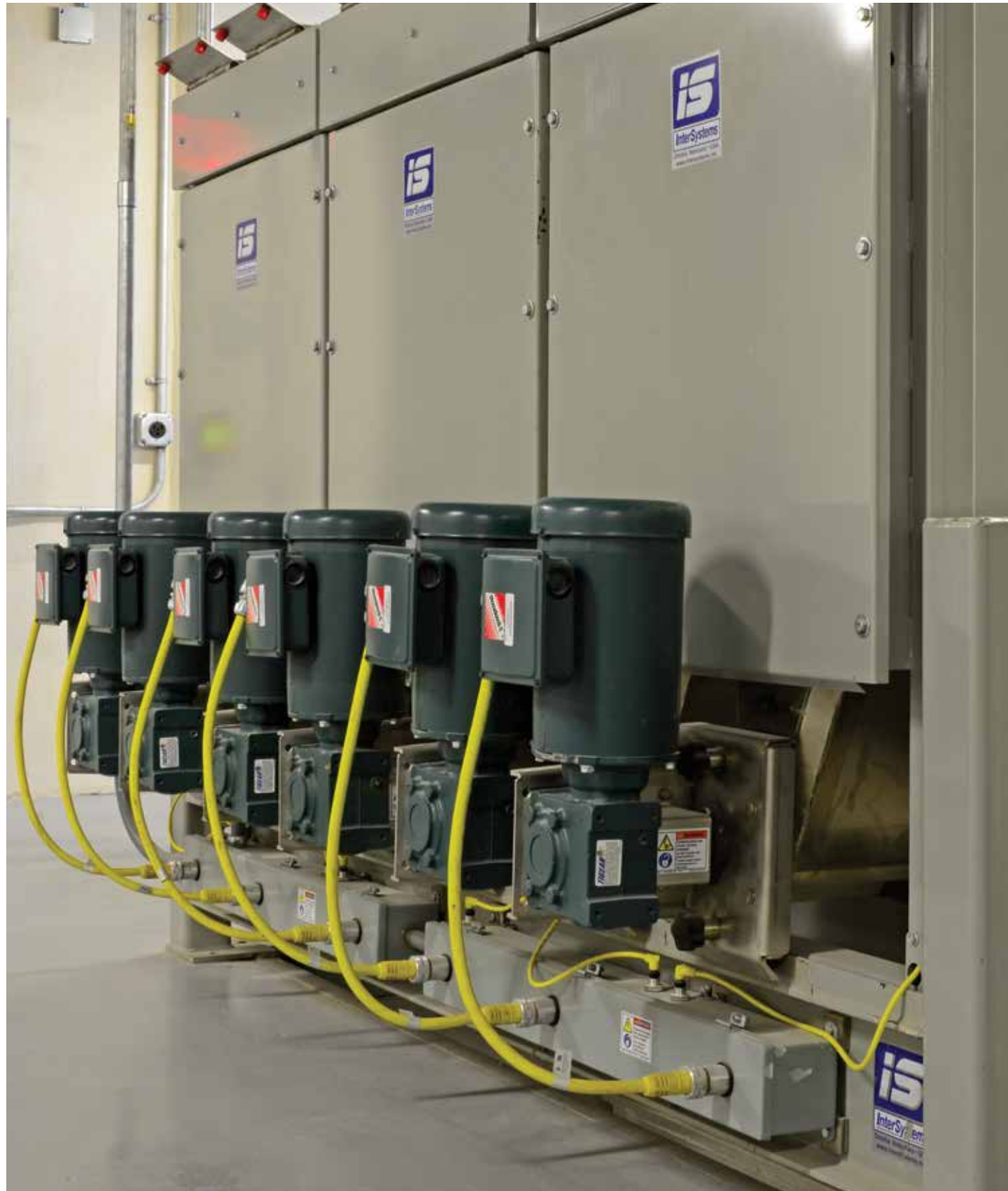
This Intersystems 12-bin micro ingredient weight loss system accurately measures and dispenses vitamins and minerals into the feed. Baldor products are standard on its equipment, like the Baldor•Reliance motors and Baldor•Dodge Tigear-2® reducers used on its microfeeders.
