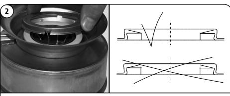
Replace any Seal Ring (Pos. 45) in the Chambers (Pos. 4, 4a, and 5a). Inner edge must face downward (see diagram). Snap Seal Ring Retainer (Pos. 65) into place. The retainer should not spin on the chamber, and the seal ring should move freely from side to side.
