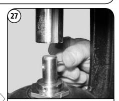
Place the Shaft Pin (Pos. 10) into the Shaft (Pos. 51).
