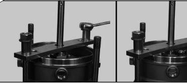
An alternative to step 21 is when the special tool 00SV2078 and two 27.5 mm Spacers (96491537) are used with two Staybolt Nuts and Washers.
