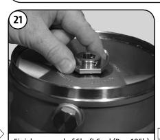
Finish removal of Shaft Seal (Pos. 105b) from Pump Head Cover (Pos. 77a). Flip the Pump Head Cover over and go to step 22.
