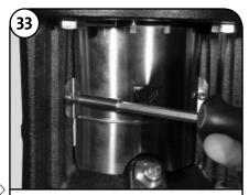
Install the Coupling Guards (Pos. 7) and the Screws (Pos. 7a). Using a Torque Screwdriver, with a slotted or a TORX® tip T20, torque to 1.5 ft.-lbs. or 2 Nm.
