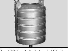
Place the Holder for Shaft, 00SV0040, in a vise. With the shaft pin inserted into the shaft, place the impeller stack into the shaft holder. Tighten vise. Using a 13 mm wrench, remove the Chamber Stack Strap Bolt (Pos. 26b), Washer (Pos. 26c), and Strap (Pos. 26a).
