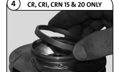
Press new Wear Ring (Pos. 49c) onto Impeller (Pos. 49a). CR, CRI, CRN, use new Impellers if eyelet of Impeller is
