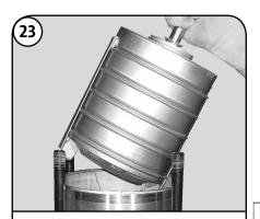
Grab the shaft and lift impeller stack out of the pump. If it is stuck, a light blow with a rubber mallet may be needed to jolt the stack free.
