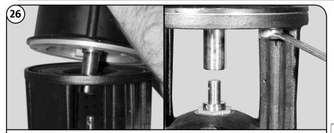
Lower motor onto Motor Stool and/or Spacer (Pos. 1), then install and tighten Motor Bolts (Pos. 28) diagonally to the proper torque.
