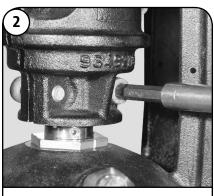
Remove the 5, 6 or 8 mm Hex Head Coupling Bolts (Pos. 9) from the Coupling Halves (Pos. 10a).
