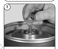
Place the Clamp Spacer (Pos. 64c) onto the shaft.
