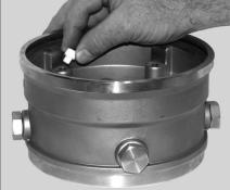
Remove the Sleeve O-Ring (Pos. 37) and the PTFE Stack Compression Springs (Pos. 60) from the Pump Head Cover (Pos. 77a).
