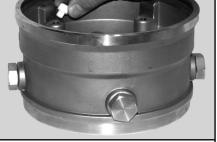
Remove Sleeve O-ring (Pos. 37) from the pump Head Cover (Pos. 77a). Then remove the PTFE Stack Compression Springs (Pos. 60a) from the Pump Head Cover.
