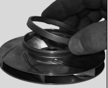
Wear Rings (Pos. 49c) can be removed on CR/CRI/CRN15 and 20 models. Impellers (Pos. 49a) use Puller 00SV2091 and Support 00SV0043 to work Wear Ring off of impeller.
