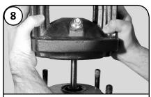
Remove the Motor Stool (Pos. 2) and Pump Head (Pos. 77) on I and N models. (Light upward blows with a rubber mallet may be required.)
