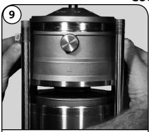
Remove the Cool-Top® assembly/Pump Head Cover (Pos. 77a). Light blows with a rubber mallet may be required to loosen assembly.
