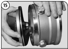
Press the plate firmly in place. Before proceeding to step 16, flip the Pump Head over; make sure the PTFE Stack "Compression Springs" (Pos. 60a) and the Sleeve O-ring (Pos. 37b) have been installed from step 1. If they have not been installed, follow the instructions in step 1 (page 9), then proceed to step 16.
