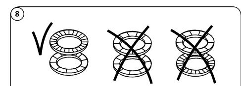
The Lock Washers (Pos. 66) come as a set. If they become separated, it is important the washers are repositioned correctly as noted in the diagram. The tabs should interlock while the serrated edges both point outward. Place the washers onto the shaft.
