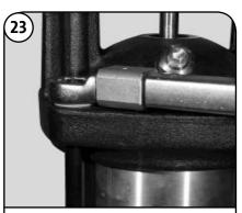
Place the Washers (Pos. 66a) over the Staybolts (Pos. 26). Then, lubricate with a light oil. Place the 24 mm Staybolt Nuts (Pos. 36) onto Staybolts and tighten diagonally to:
