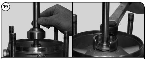
Use specialty tool, 00SV2107, a 41 mm Deep Socket, or an Open Ring Spanner to loosen.
