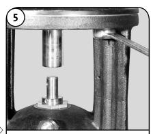
Remove the 9/16" Head UNC 3/8" or 3/4" Head UNC 1/2" Motor Bolts (Pos. 28) and lift the motor off the Motor Stool (Pos. 2).
