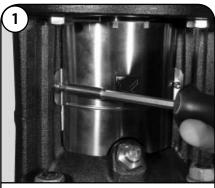
Using a slotted Screwdriver or TORX® tip T20, remove Coupling Guard Screws (Pos. 7a). Then, remove the Coupling Guards (Pos. 7).
