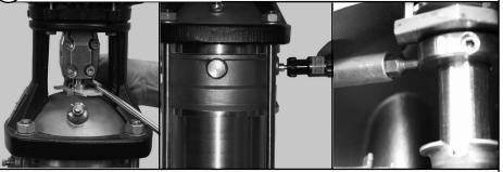
Using a screwdriver, lift the Shaft upward. Insert <u>two</u> of the Spacer tools between Shaft Seal Collar and Hex Nut. Insert a 2.5 mm allen wrench through one of the lower vent port holes and torque the lower inboard seal securing screws to 2.0 ft.-lbs./2.5 Nm. Remove allen wrench and replace plugs (Pos. 23a) into the Pump Head Cover (Pos. 77a). Remove only <u>one</u> Spacer. Then, tighten and torque the Coupling bolts to values in step 29.
