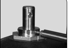
Pushing down on Shaft Seal collar (do not push down on Hex Nut), lower the new Shaft Seal (Pos. 105) over the Shaft. Use specialty tool, 00SV2107, a 41 mm Deep Socket, or an Open Ring Spanner to tighten to 26 ft.-lbs. or 35 Nm. Push the Shaft all the way down (for Tandem Seal models you must continue to apply downward force), then tighten the three 2.5 mm Shaft Seal Securing Allen Screws torque to 2 ft.-lbs. or 2.5 Nm.
