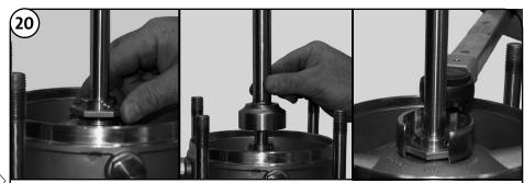
Slide the Inboard Seal (Pos. 105b) down the shaft and thread into the pump head. Use specialty tool, 00SV2107, a 41 mm Deep Socket, or an Open Ring Spanner to torque the Inboard Seal to 26 ft.-lbs./35 Nm.
