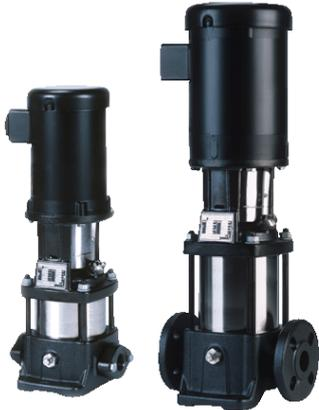
Vertical, multistage centrifugal pump with suction and discharge ports on the same level. The pump head and base are in cast iron. All other wetted parts are in stainless steel (EN 1.4301)(AISI 304)
