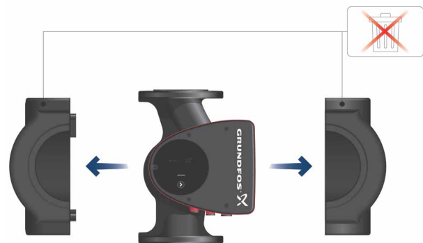
Fig. 3 Fitting insulating shells to the pump
