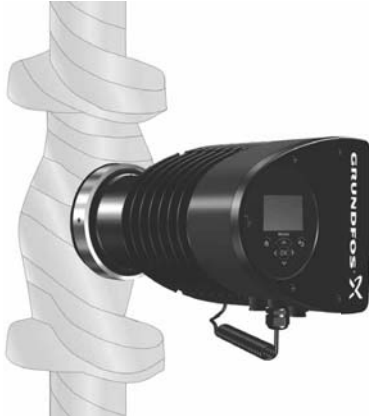
Fig. 14 Insulating the pump housing and pipe
