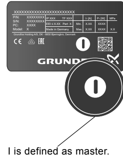
Fig. 52 Identify the master pump on a twin-head pump
