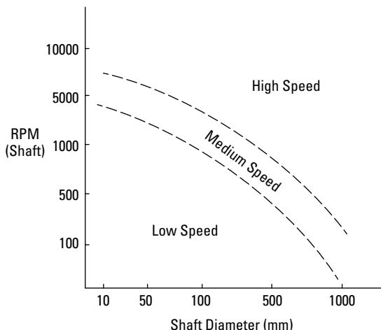
Fig. 3. Seal surface speed selection guide.
