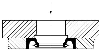
**Fig. 7. Seal Installation with an end plate.**
