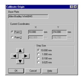
5. Click the movement arrows to move the pen until it is over the "crosshair" located in the upper left area of the base plate. Use your finger to lightly press the pen down. When the pen tip drops into the pin hole located in the "crosshair", then the first point has been calibrated correctly.
