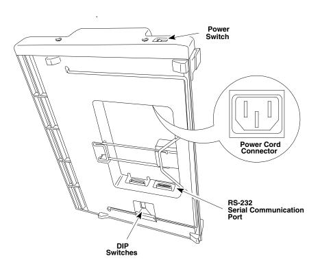
**2.** Verify that the plotter DIP switches are set as shown below. The switches are located on the bottom of the plotter.
