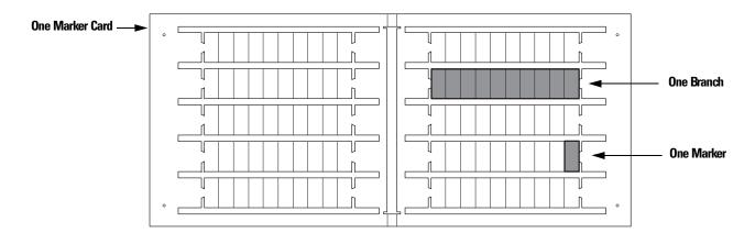
Note: Use thumbs and index fingers to apply pressure to "snap" the markers free. Never twist the markers to break them free. Twisting will result in uneven breaks.
