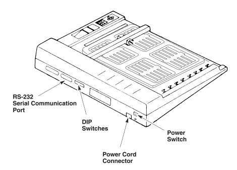
**2.** Verify that the plotter DIP switches are set as shown below. The switches that must be on (up position) are indicated by a red mark on the end.
