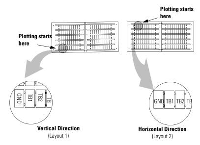
Plotting always starts in the upper left corner of the marker card when you are holding it so that the marking is readable. This results in a different starting point for vertical (Layout 1) and horizontal (Layout 2) plotting.
