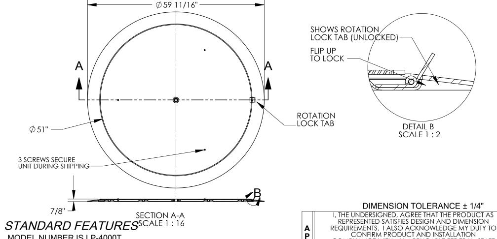
MODEL NUMBER IS LP-4000T CAPACITY IS 4,000 LBS USEABLE DIAMETER IS 51" OVERALL DIAMETER IS 59 11/16" OVERALL HEIGHT IS 7/8"
