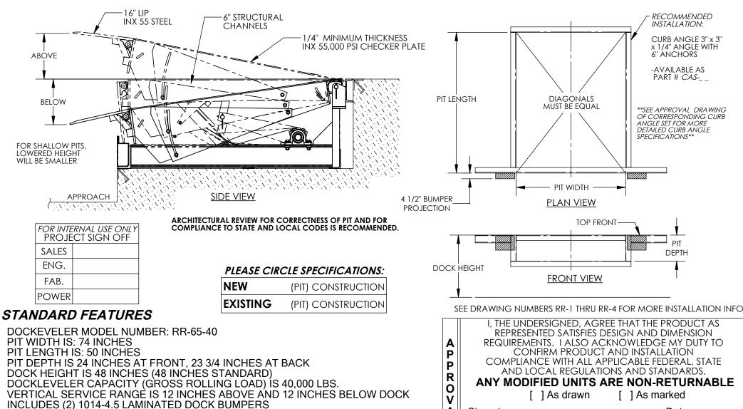
ALL STRUCTURAL STEEL CONSTRUCTION WELDING MEETS AWS. DESIGN, ENGINEERING, AND FABRICATION COMPLIES WITH OSHA & ANSI MH30.1 -INSTALL TO MEET ALL APPLICABLE STATE & LOCAL CODES FOR YOUR AREA!
