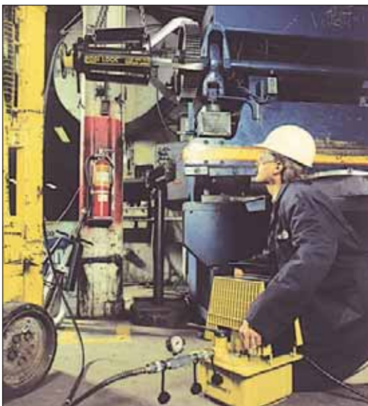
◀ An EPHR-116, 50-ton hydraulic Posi Lock® puller easily removes the main drive gear from this metal forming brake press.
