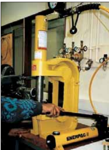
◀ A-310 Arbor Press used for compacting powder at 10 tons.
