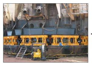
To prevent back pressure and to increase cylinder retraction speed, when using long hoses, the Enerpac HC7300 range of hoses with increased internal diameter is the best choice.
