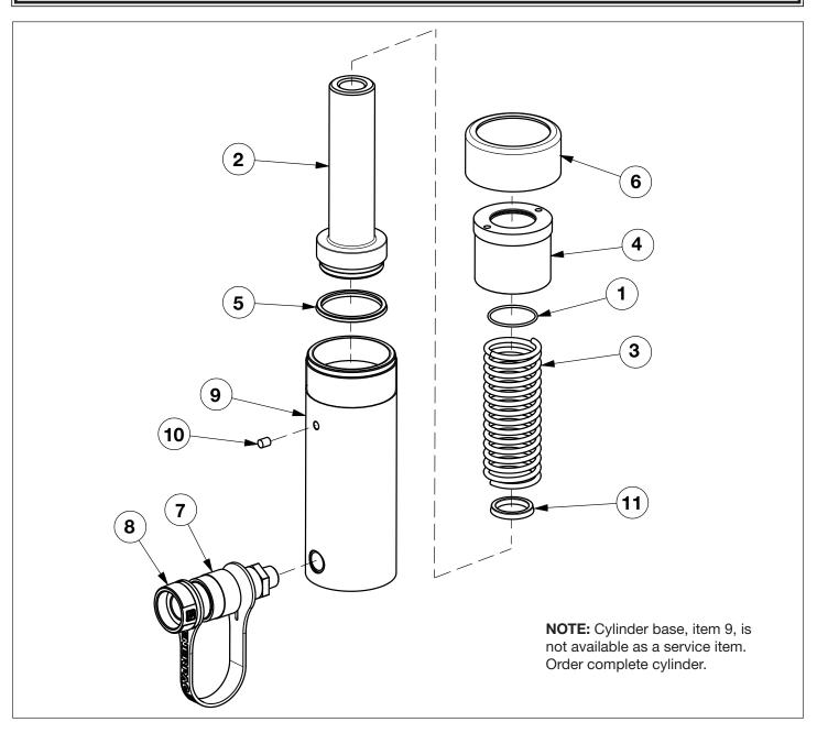
**WARNING** STOP RINGS ON RCH MODELS ARE SPRING LOADED! If not contained during disassembly, spring and stop ring could cause personal injury.
