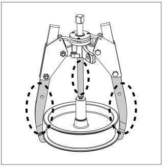
Figure 8, Checking for Deformation
