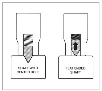
Figure 4, Retractable Point (Models SGM10 and SGM20)
