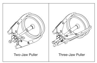
Figure 7, Pulley Removal (typical)
