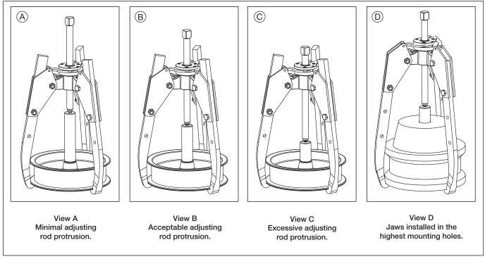
Figure 6, Jaw Mounting Positions and Adjusting Rod Height
