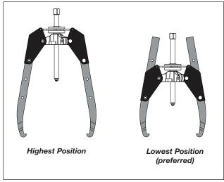
Figure 5, Jaw Mounting Positions (typical)
