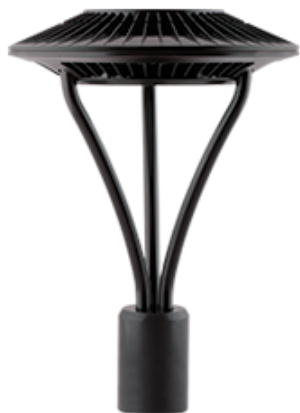
High output LED pole top area light with IES type V circular distribution. Wide and uniform 360 degree pattern ideal for large outdoor areas such as parking lots, corporate parks, and retail settings. Color: Bronze Weight: 21.8 lbs
