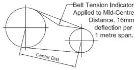
As a general rule the midpoint of the applied force should be at the midpoint of the shaft and it is good engineering practice to mount the motor pulley with hub and locking screw at the shaft end.
