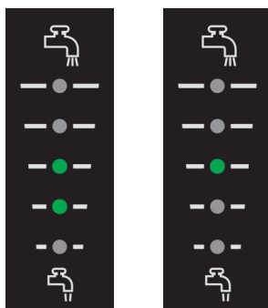
Fig. 13 SCALA2 outlet pressure indication
