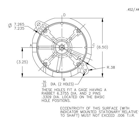
"FAH" .452/.442 X 1.34 LG. 1.41 .19 -1.32 FULL FLAT MAX. 5.61 6.375 6.370 .5000 .4995 — - "E" LEADS "ZC" LONG WITH "ZE" BWS REF. .63 → - .500-14 CND. THRD. FACE RUNOUT (WITH INDICATOR MOUNTED STATIONARY RELATIVE TO SHAFT) MUST NOT EXCEED .006 T.I.R.
