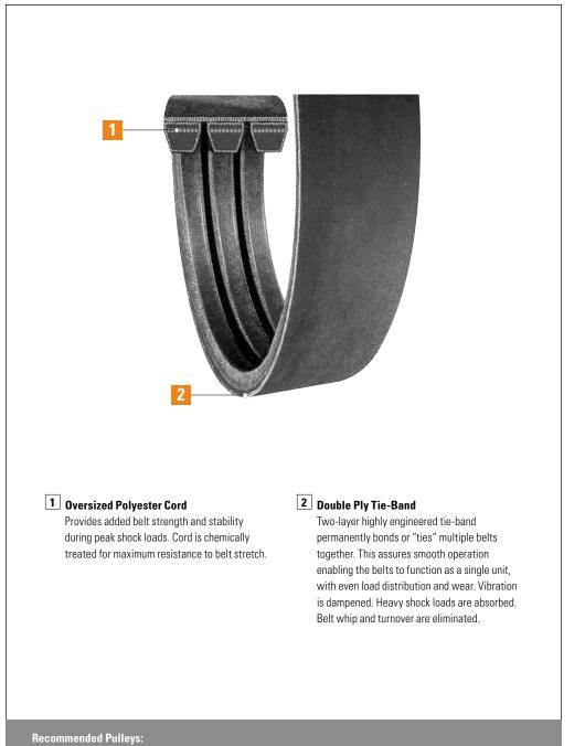
Hi-Cap Wedge – QD, Taper Bushed, or MST (3V, 5V, 8V)
