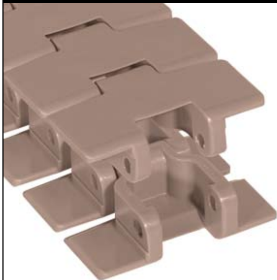
Photo shows LPC279® TableTop® Chain with Low Pin Centerline molded in Low Friction (LF) material.
