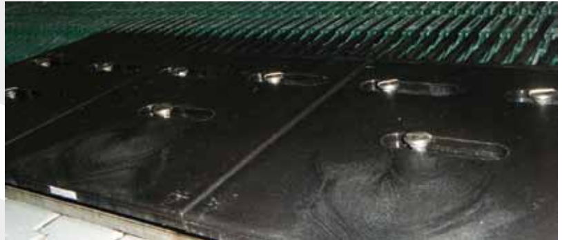
Finger-tighten Screws Across Entire Conveyor Width
