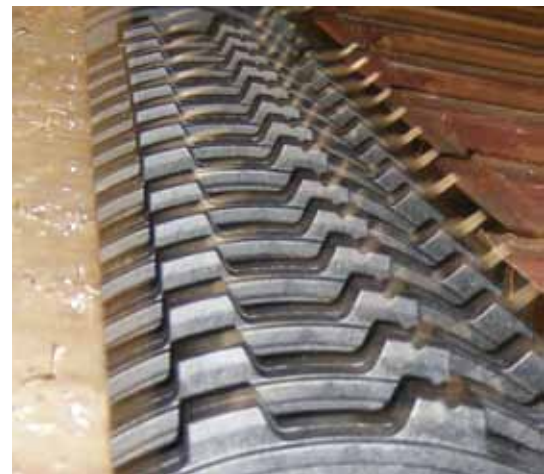
Properly Installed Sprockets with Timing Mark in Alignment
