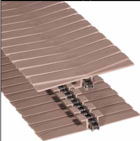
Photo shows 3873 TAB TableTop® Chain with top plates molded in Low Friction (LF) material on Stainless Steel (SS) base chain.
